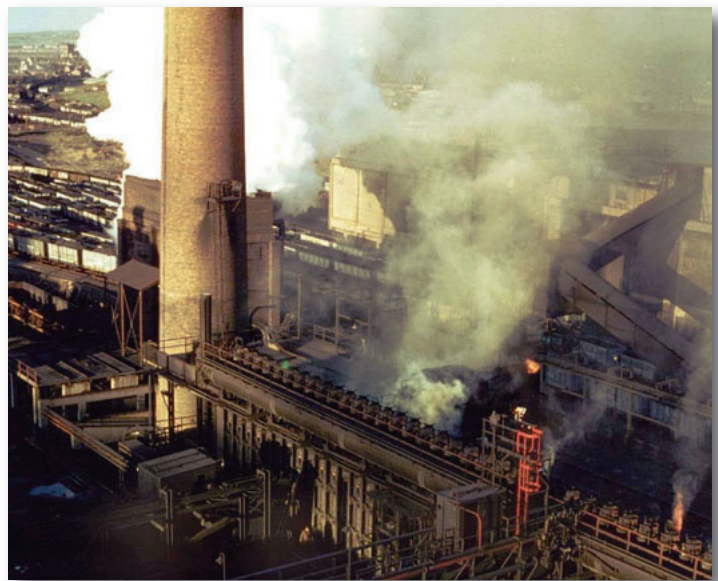
Pictured above: Coke ovens charging at the former Bethlehem Steel plant in Lackawanna, New York.
