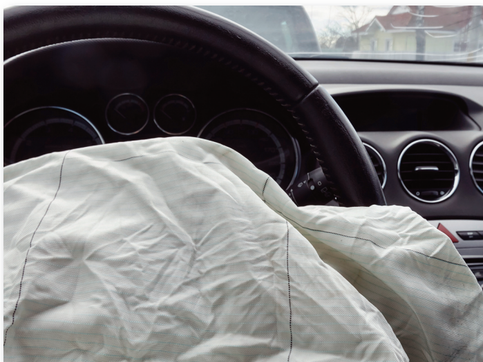
Pictured above: Dislodged airbag from a car's steering wheel. The defective design of Takata air bags caused them to explode on impact.
